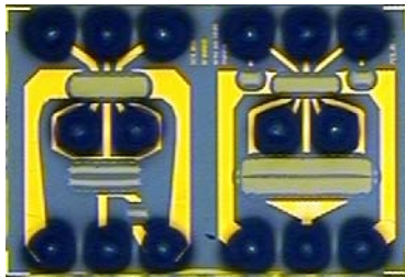
Fig. 12. Bottom side of dual high band SAWs in WLP format. Source: RFMD
