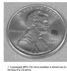
Fig. 11 3 \times 3 \text{mm}^2 MEMS Oscillator [20]
