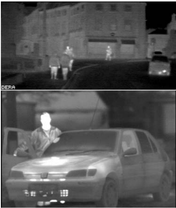
9 High resolution pyroelectric images: 256 \times 128 pixels (above), 384 \times 288 pixels (below) (courtesy UK Defence Evaluation and Research Agency, 1998)
