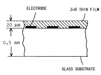
Fig. 9. Cross-sectional view of a 58-MHz SAW filter using ZnO thin film on glass.
