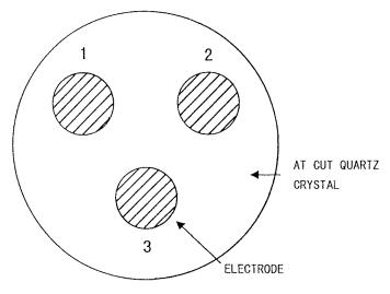
Fig. 5. Electrode arrangements on a quartz crystal "Uni-wafer."
