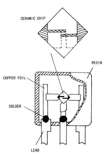
Fig. 10. The physical configuration of a 57-MHz double-mode ceramic resonator for video IF.
