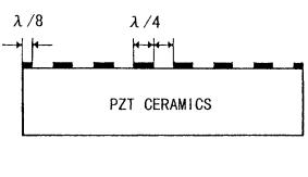
Fig. 11. (a) Electrode arrangements of a 40-MHz BGS wave resonator and (b) cross-sectional view of the resonator.
