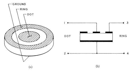
Fig. 3. (a) The physical configuration of a "Transfilter" and (b) its symbolic circuit.
