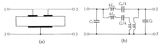
Fig. 6. The symbolic circuit of a crystal filter using multi-energy trapping vibration modes and (b) the equivalent circuit.
