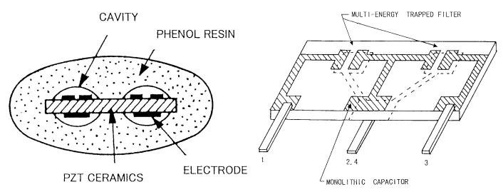
Fig. 7. The package of a 10.7-MHz ceramic filter.
