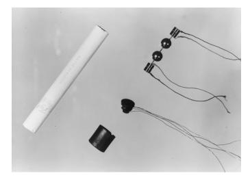
Fig. 1. Inner structure of a 455-kHz mechanical filter using steel balls and Langevin-type transducers with barium titanate.
