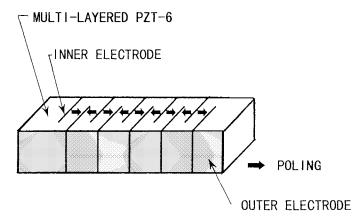
Fig. 12. The physical configuration of a 450-kHz ceramic resonator using multi-layered PZT ceramics.
