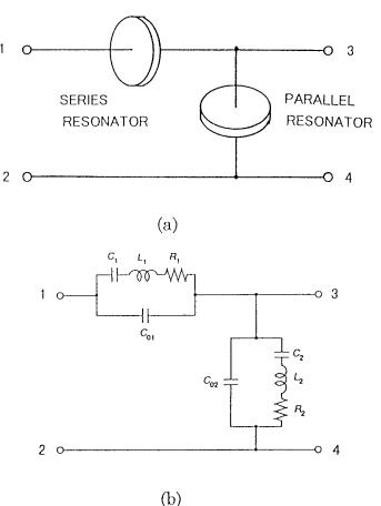
Fig. 2. (a) An L-section of a ladder-type ceramic filter with ceramic resonators in the series and parallel branches and (b) the equivalent circuit.
