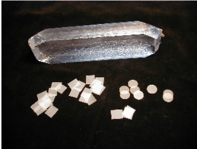
Figure 46: Slab of Large Cultured Quartz Crystal, Shown with Rectangular and Circular Blanks (Personal photograph of Richard J. Thompson, Jr. Reprinted by permission. thompso@strose.edu)
