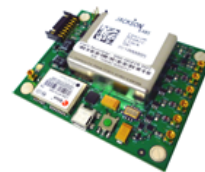
Fig. 71. Microsemi CSAC & Physics Package. Photo Credit: Microsemi & Symmetricom.
