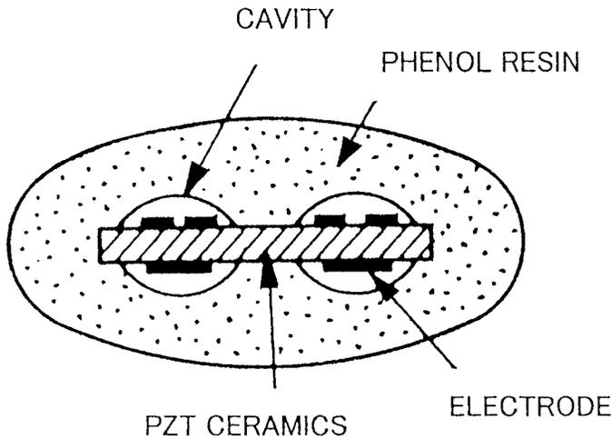
Fig. 7. The package of a 10.7-MHz ceramic filter.
