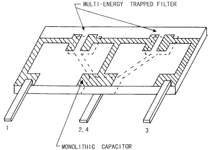
Fig. 8. The physical configuration of a monolithic ceramic filter with a monolithic capacitor.
