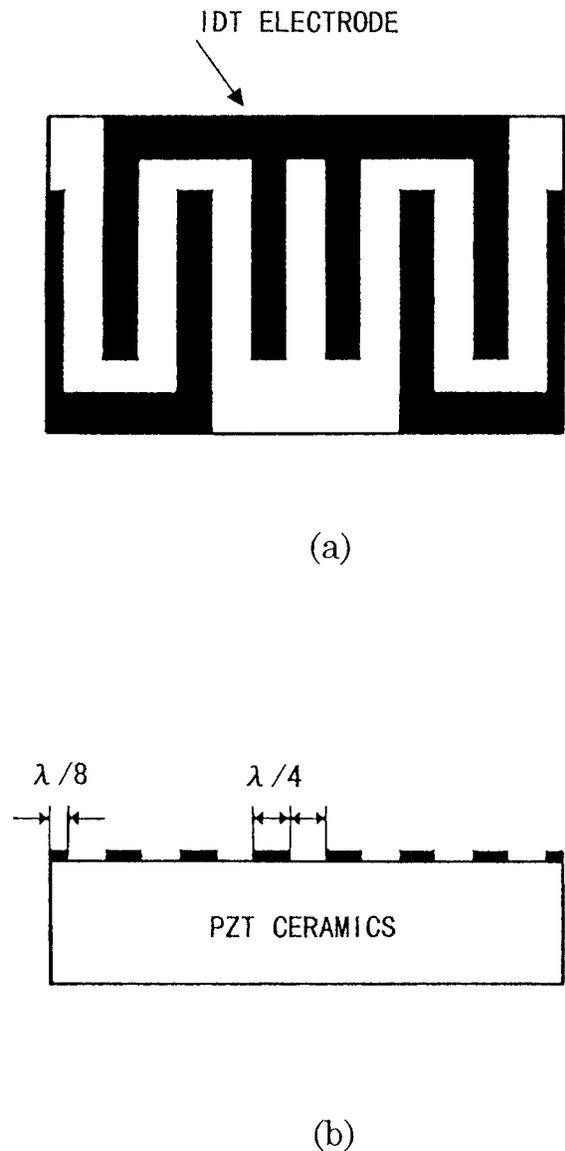
Fig. 11. (a) Electrode arrangements of a 40-MHz BGS wave resonator and (b) cross-sectional view of the resonator.
