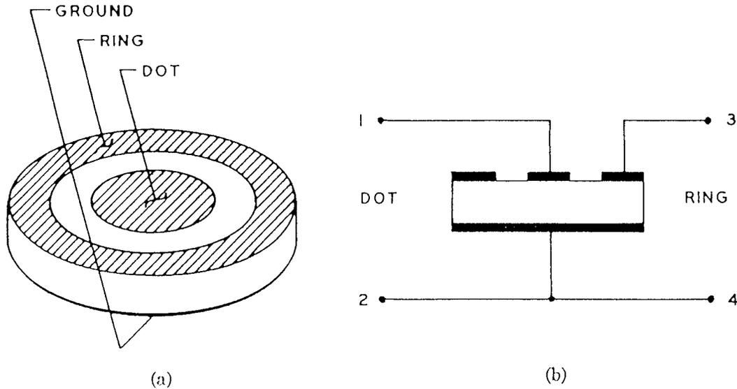
Fig. 3. (a) The physical configuration of a "Transfilter" and (b) its symbolic circuit.
