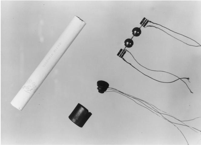
Fig. 1. Inner structure of a 455-kHz mechanical filter using steel balls and Langevin-type transducers with barium titanate.
