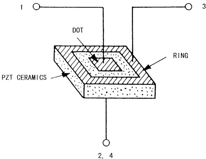
Fig. 4. The physical configuration of a 455-kHz ceramic filter.
