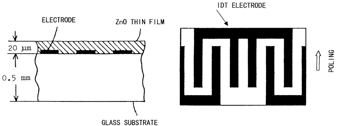
Fig. 9. Cross-sectional view of a 58-MHz SAW filter using ZnO thin film on glass.
