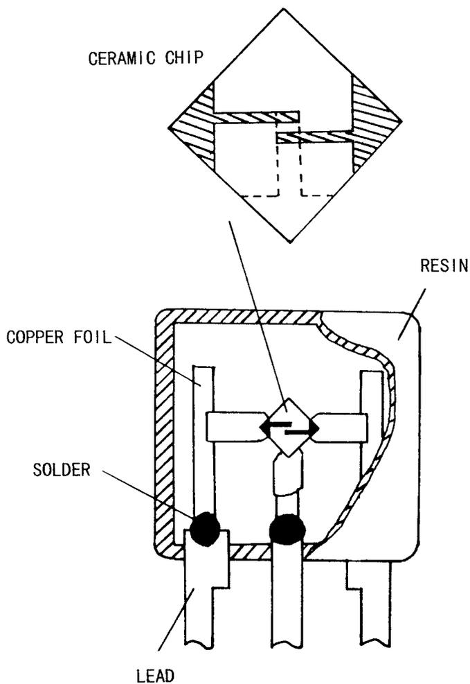
Fig. 10. The physical configuration of a 57-MHz double-mode ceramic resonator for video IF.
