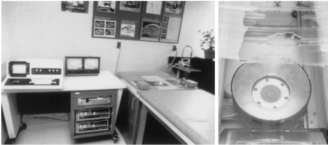
Fig. 5. Automated whole breast imaging system manufactured by Life Instruments Corporation in 1983. This system was a prototype employing a hybrid PVDF cone annular array transducer. This scanner was used in a clinical study of over 1700 women at Women's College Hospital, Toronto. The transducer is shown at the right.
